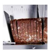
The slice thickness lies between 3 and 30 mm and can be adjusted via keys during operation. Three save keys enable quick toggling between the three slice thicknesses that can be programmed individually.
