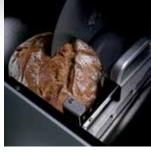
An optimized rotation speed lowers the operation noises and ensures a smooth machine running, better slicing results and less generation of heat.
